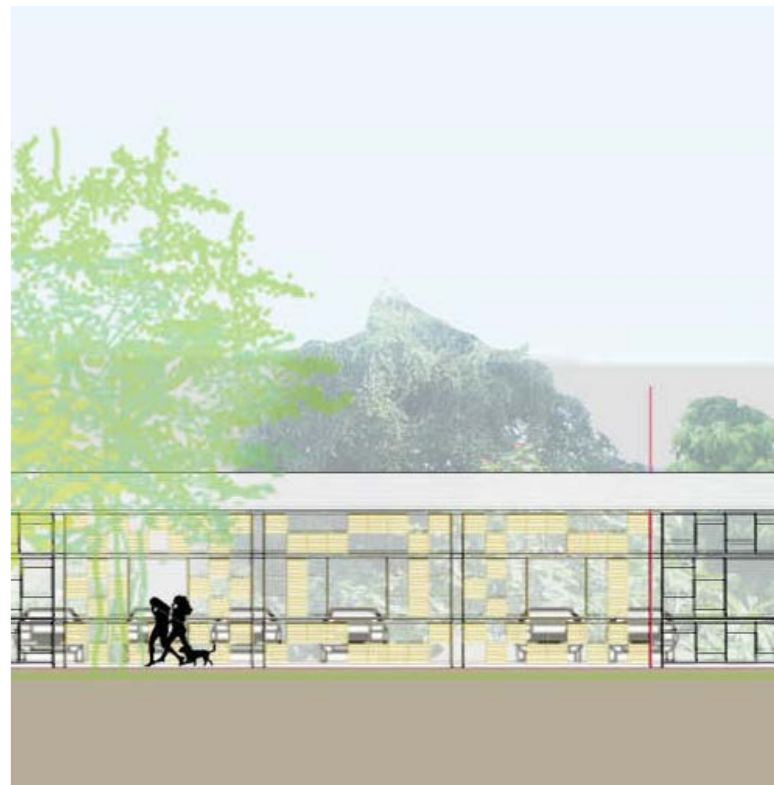
THE EXISTING OPAQUE PLASTERED WALL IS REPLACED BY A 4m HIGH TRANSPARENT METAL GRILLWORK SCREEN. ALL VEHICLES PARK BEHIND THIS. AS GMC IS AN IMPORTANT LAND-MARK BETWEEN 2 MAJOR GOAN CITIES, THIS SCREEN ALSO SERVES AS AN INTERESTING URBAN ART WALL.
